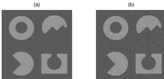
Figure 1: (a) artificial gray level image (b) adding i.i.d. Gaussian noise on the image in (a)
